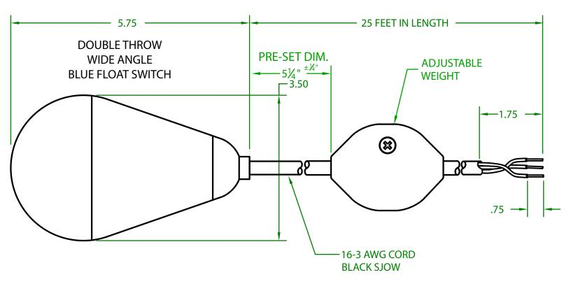
OPERATING ANGLE: SWITCHES @ 45° ABOVE AND 45° BELOW HORIZONTAL. @ 45° ABOVE HORIZONTAL: (RED IS CLOSED / WHITE IS OPEN) @ 45° BELOW HORIZONTAL: (NORMAL POSITION) (RED IS OPEN / WHITE IS CLOSED)
